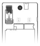
Remove the battery cover and insert the memory card with the gold-coloured contacts facing down.
